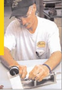
Quality control is top priority at Magnus. Every broadhead must pass a precision spin test before it is shipped.
